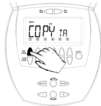
Fig 16b – Press and release the Channel 1 ON/DIM button on the Primary Controller . "TA" which stands for "Transmit ALL data" will be shown next to "Copy".
