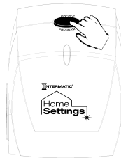
Fig 9c – Set the desired light level by pressing the PROGRAM button on the module. Release the INCLUDE button on the controller when the light level is set.
